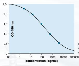
Example of typical calibrator curve using a 4 PL (4 Parameter Logistics) curve fit.
