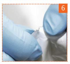
Tear the aluminium envelope open at the notch. Once the device has been taken out of the envelope its stability is of short duration, especially in a humid environment.
